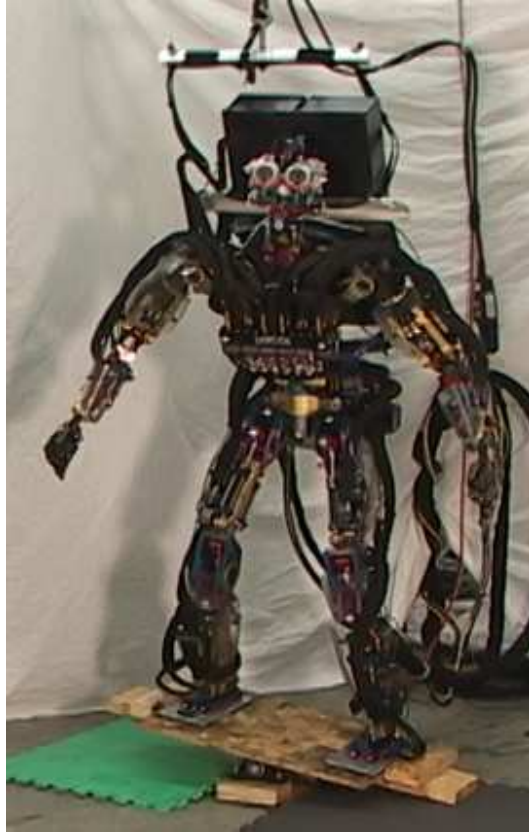
Figure 1.2: The Sarcos Primus humanoid on a seesaw.
